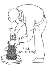
Figure 35-C. Slump Test (Full-Overflow)
